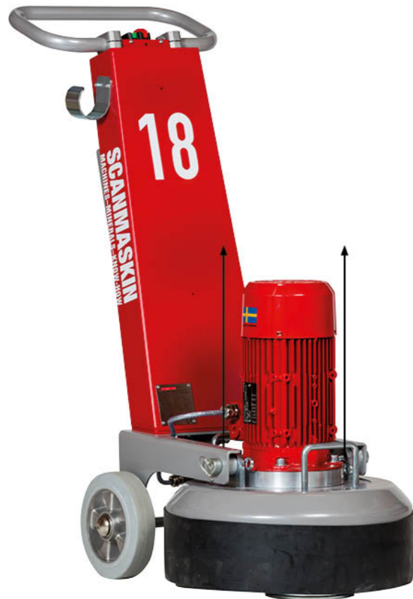
Figure 3-2 Lifting points Scanmaskin 18
