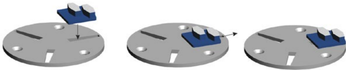
Figure 4-4 How to fit the diamond segments on the Scan-On plate
