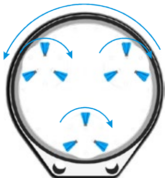
Figure 4-1 Illustrates the rotation of the grinding heads versus the gear barrel.
