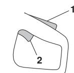
When the grip on the handle is released, both the throttle and throttle lockout return to their original positions. In this position, the machine will stop and the throttle will be locked, while the water valve returns to closed position.
