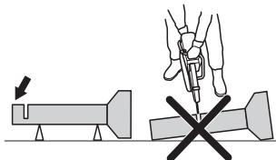
If the pipe is allowed to sag and close the cut, the blade will be pinched in the kick back zone and a severe kick back might develop.
