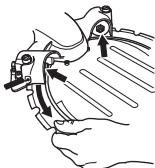
**CAUTION!** The machine should be upright. If the machine lies on its side the weight of the blade makes it difficult to make a correct adjustment. Incorrect adjustment can result in damage to the blade. If the blade rotates slowly or stops, stop cutting immediately and trouble shoot.
