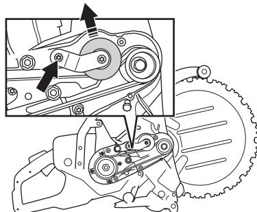
**NOTICE!** Make sure that both belt pulleys are clean and undamaged before a new drive belt is fitted.
