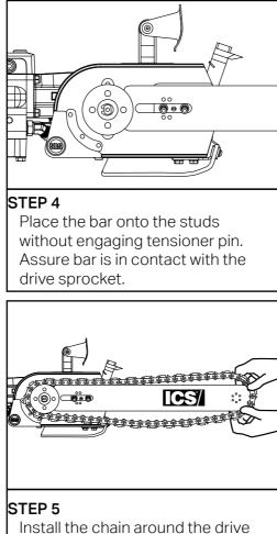
Install the chain around the drive sprocket and then around the nose sprocket before inserting into the bar groove.
